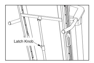
Hold the metal frame firmly with both hands, and lower it to the floor. CAUTION: To decrease the possibility of injury, do not lower the frame by gripping only the plastic foot rails. Do not drop the frame to the floor. Make sure to bend your legs and keep your back straight.
